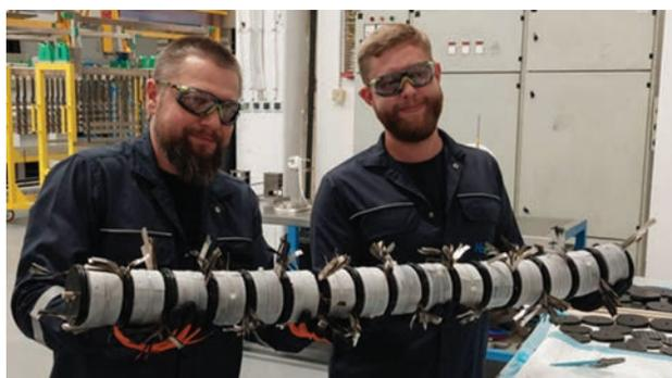
Figure 2c: A stack of rolled electrodes – Photo@H<sub>2</sub>Pro.
